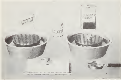
11-17. The equipment and supplies needed to lap seals and valve plates. Note the magnifying glass used for inspection. (Norge Sales Corp.)
